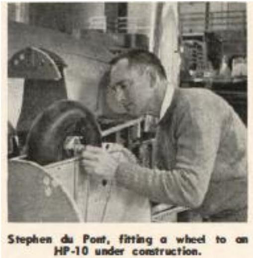
Stephen du Pont, fitting a wheel to an HP-10 under construction.
