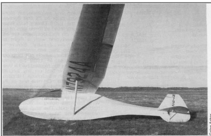
This sailplane, the Schultz Nucleon, was built in 1954 and had a span of 46 feet with aspect ratio of 16 utilizing an NACA airfoil NACA 65(2)-415, 64(1)-A212. Empty weight was 345 lbs with gross weight 535 lbs. The structure was single strut braced all-wood wings, steel tube/fabric wings and braced tail. L/D estimated at 22 (47 mph) and minimum sink 3.3 fps at 43 mph. The wing was built of
