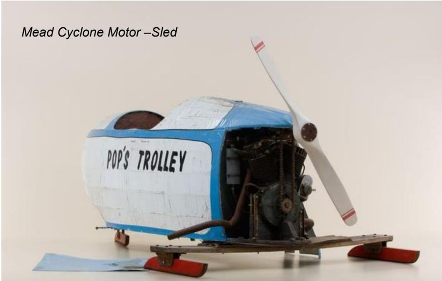
← From the Harley-Davidson Museum in Milwaukee, the Mead Cyclone Motor-Sled, "Pop's Trolley." These ice sleds could be built from a kit, circa 1930. "Pop's Trolley" was a Mead Cyclone motor sled powered by a 1925 Harley-Davidson engine.
